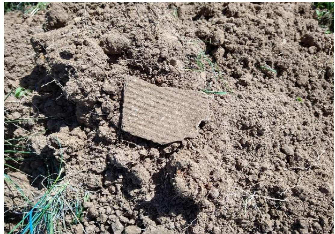
Photo 4: View of asbestos fragment observed in the fill in Pit 8.
